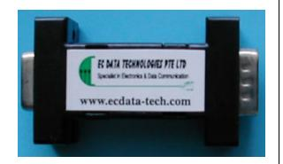
The ECD232TTL is designed to convert the RS-232 level signals into TTL/CMOS level signals. The unit allows you to connect a TTL device, such as the serial port on the micro-controller, to the serial port of the PC. The conversion circuit is housing inside the DB9 adaptor housing and the power is supplied from the micro-controller board.
