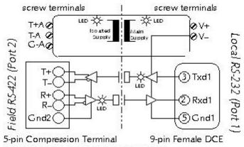
Note: When ordered connector type is configurable
