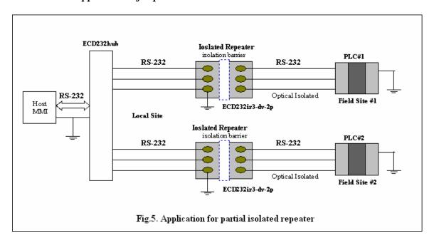
Here is a common installation of the ECD232ir3 with 2-port optical isolation. A small power supply with 2.5Kv isolation powers the two ECD232ir3 units. Since all two host RS-232 circuits share a common ground within the computer, any concern about devices
